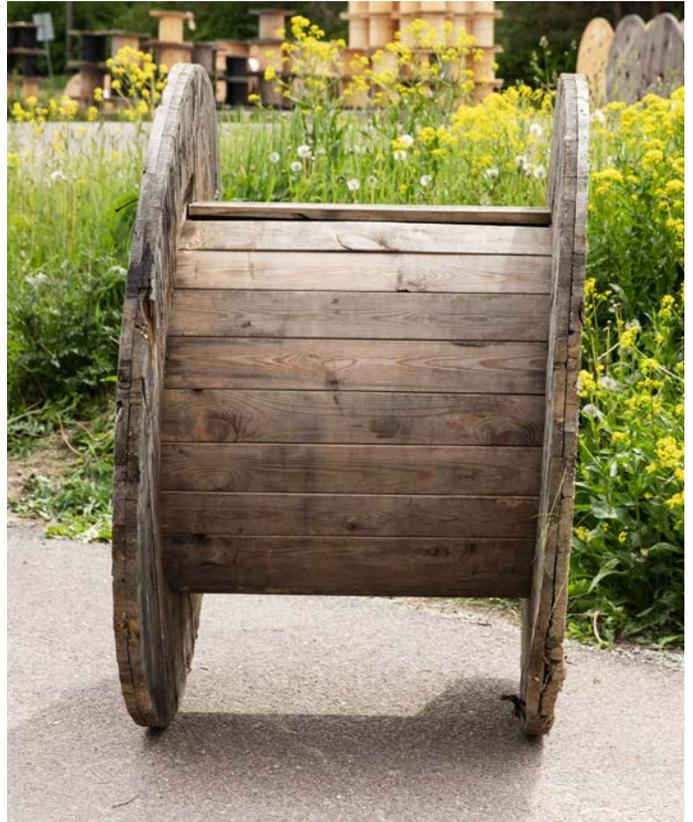
**B** The drum flange is inclined.
