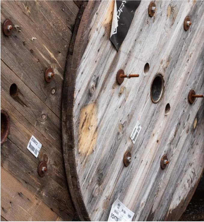
**E** The metal elements of the drum are defective or missing.
