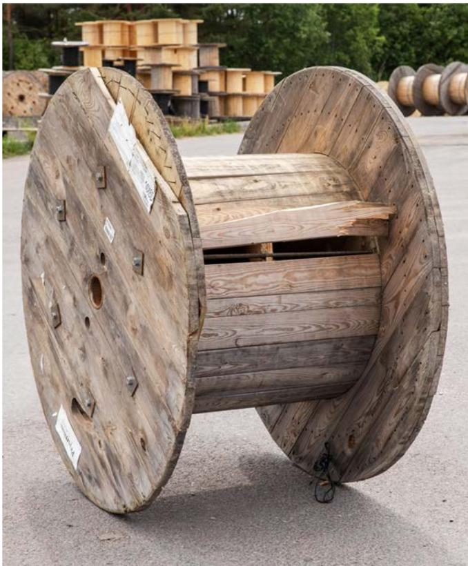
**C** Boards are missing or broken.
