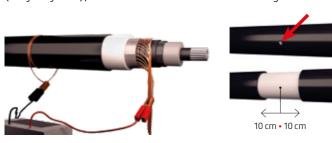
Sheath current can also be identified with a megger. The formula for sheath current is then:
