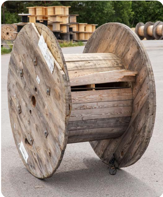
C Boards are missing or broken.
