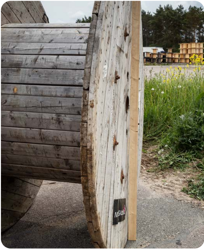
A The drum flange is bent.
