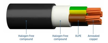
**XPK-HF C-Pro** is a 1 kV halogen-free flame-retardant power cable for fixed indoor and outdoor installations. The cable is suitable for building installations, residential construction, industrial installations, and data centres. The cable meets fire performance Cca-s1,d1,a1 and is suitable for use in buildings with a high fire risk. In the event of fire, smoke generation is low and transparent which facilitates evacuation; smoke is also not harmful to electronic equipment.
